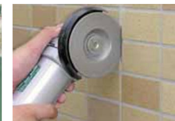
▲ For grooving tile joints etc.
