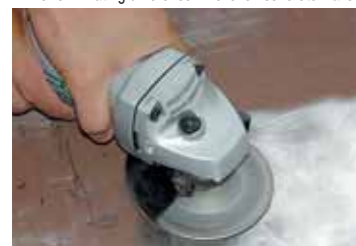
▲ For removing mill scale
