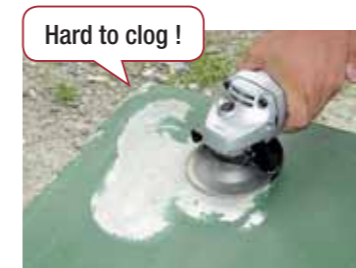
▲ For removing elastic film
